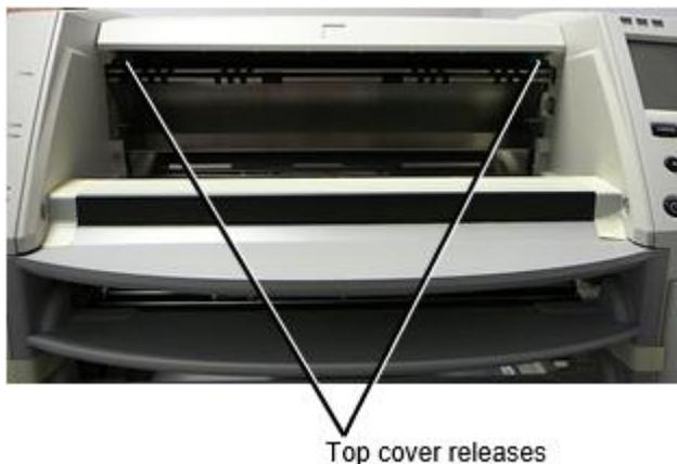
**NOTE:** The top cover is spring-loaded. Place your hand lightly on the top cover before pressing one of the releases to prevent it from opening too quickly.
