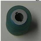
7. Orienting the pick tire with the notched side first, slide the pick tire all the way on to the spindle, making sure you align the notches with the spindle pins.
