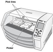
Using PLATEN ROLLER Cleaning Wipe provided with the imager's cleaning kit, wipe around each pick tire with the cleaning wipe. The cleaning wipe may become discolored.
