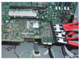
3. Disconnect the SATA cables by squeezing the release latch and pulling the cables from the RAID Adapter.
