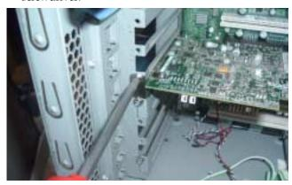
Pull the RAID Adapter from the motherboard slot far enough to disconnect the battery cable from the RAID Adapter before completely removing the card.
